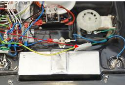
3. Remove the 2 nuts and washers holding the motor.
