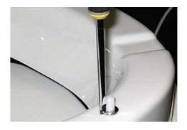
3. Pull off the handle for the heat regulation on top. Lift the top part straight up.
