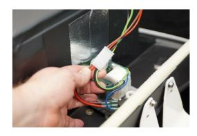
2. Loosen the 4 screws holding the mixer motor (gear box).
