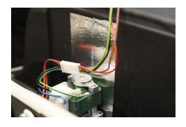
2. Disconnect the quick release contact to the bottom heater.
