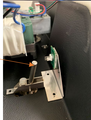
Compost sensor Operates by the compost level in upper chamber, when level reaches upper rake the sensor activates by a small magnet through the axle
