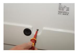
Remove the fastening in the front with a slotted screwdriver.
