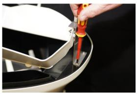
Remove the torxscrew (T15) in the center of the rear bracket. It's partly covered by the foam gasket. Try to avoid damaging the gasket.
